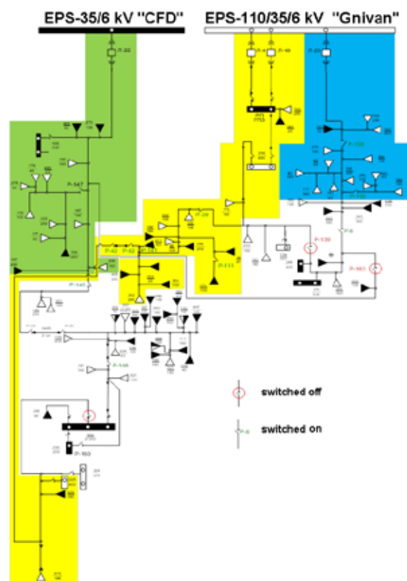
Fig. 2. The distribution network with selected unconditional attractors of feeders and a boundary zone
