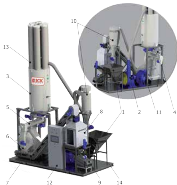
Fig. 4. Technological scheme of the mini-line production of fuel pellets from energetic willows: 1 – receiving hopper; 2 – hammer crusher; 3 – intermediate bunker; 4 – dispenser; 5 – mixer; 6 – press granulator GT-304 D; 7 – belt conveyor; 8 – cooler GTO-0.6; 9 – vibration sieve GTII-1; 10 – cyclone; 11 – fan; 12 – control panel; 13 – filters; 14 – platform
