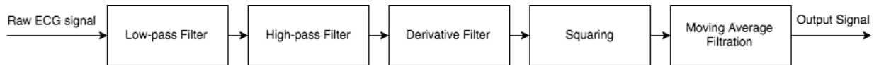
Fig. 1. Common block-diagram of ECG-signal filtration tract. Consist of: low-pass filter, high-pass filter, derivative filter, signal squaring, moving average filtration stage
